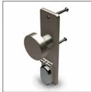
Short Plate with cylinder hole GSV-No. 6657 ZK/1-75 - Stainless Steel plate - Fixed Knob stainless Steel - Spring Loaded Folding Cover stainless Steel - Through Fixing bolts
